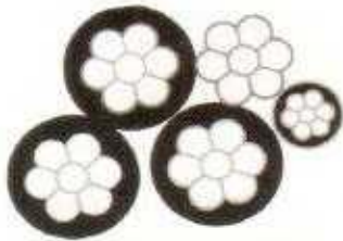
Cross Sectional view Aerial Bunch Cables
